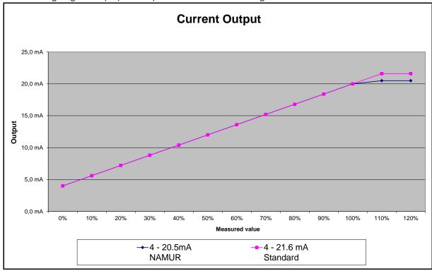
Figure 2: Current Output as NAMUR or Standard
