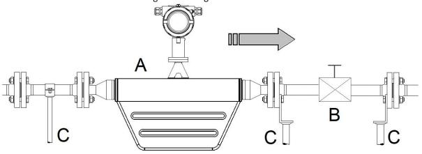
Flowmeter installation: A = sensor, B = valve, C = pipe clamps and supports
