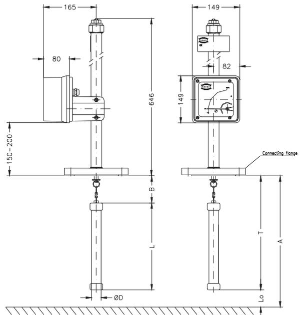
8.1.2 Indicator housing made of stainless steel
