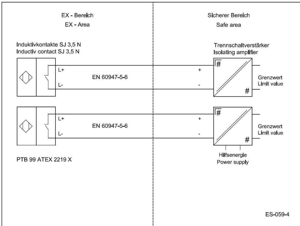
9.5 Wiring diagram for KEM 1 and KEM 2 micro switches
