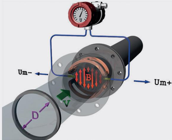
An electrically conductive medium flowing through an orientated magnetic field, in accordance to Faraday's law of induction, will induce a voltage proportional to the mean flow velocity rate and hence the volumetric flow.
