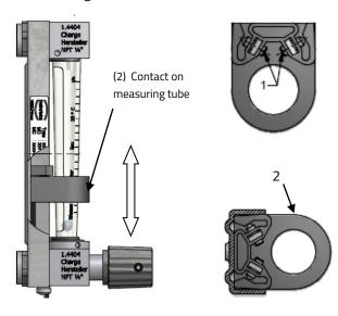
The limit switch (ring form) can be adjusted up and down the measuring tube. It is fixed via two screws (1) at the back wall of the instrument.
