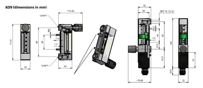
The M4 threaded pins are only an integral part of the delivery if the option "Wall Mounting" has been selected.
