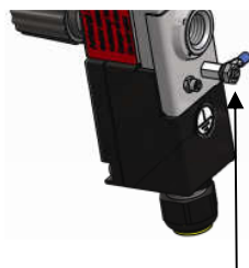
Grounding at variant with an add-on terminal case.
