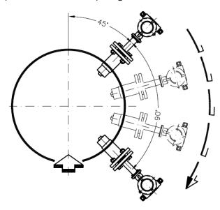
In order to stay within the indicated accuracy, the installation must be performed according to EN 29104 "Measurement of Fluid Flow in Closed Conduits – Methods of Evaluating the Performance of Magnetic-Inductive Flow meters." Based on this standard, the minimum straight run of pipe ahead of the inlet must be 10 pipe diameters (> 10 x DN) and 5 pipe diameters following the outlet (> 5 x DN) [DN = nominal diameter of pipe].
