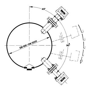
In order to stay within the indicated error limits, the installation must be performed according to EN 29104 "Measurement of Fluid Flow in Closed Conduits — Methods of Evaluating the Performance of Magnetic-Inductive Flowmeters." Based on this standard, the minimum straight run of pipe ahead of the inlet must be 10 pipe diameters (>  $10 \times DN$ ) and 5 pipe diameters following the outlet (>  $5 \times DN$ ) [DN = nominal diameter of pipe].
