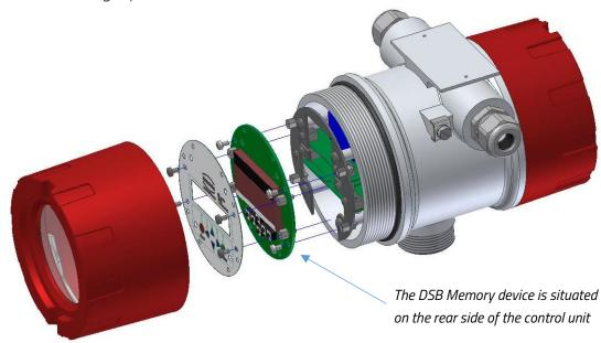
Removal and exchange of the BE4 Control unit:
