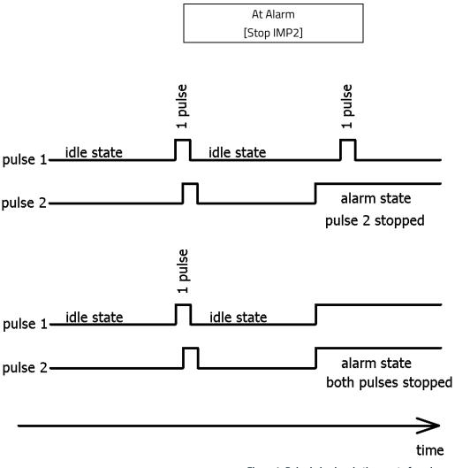
Figure 4: Pulse behaviour in the event of an alarm
