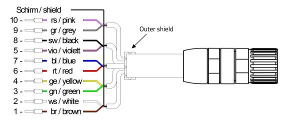
The outer shield is connected to the terminal box cable gland at one end, and the connector's outer-case at the other end. The inner shields of the wire-pairs are connected to each other (drilled together) and connected to the "Schirm / Shield" terminal in the junction box.
