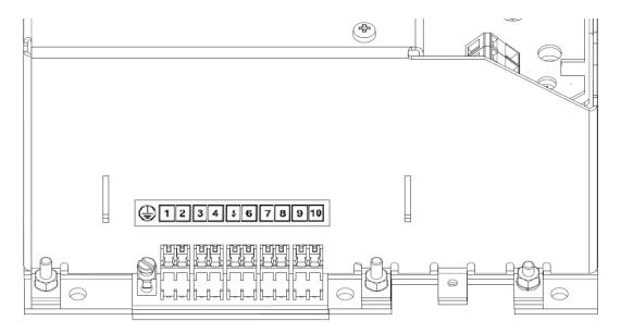
The connected cable requires a strain relief near the terminal blocks
