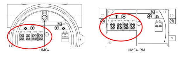
Output Signals shown in Ex-ia type of protection
