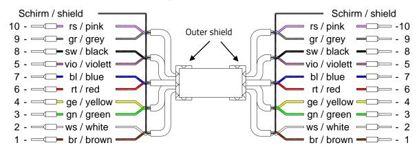
The outer shield is connected to the terminal box cable glands at both ends, The inner shields of the wire-pairs are connected to each other (drilled together) and connected to the "Schirm / Shield" terminal in the terminal box.
