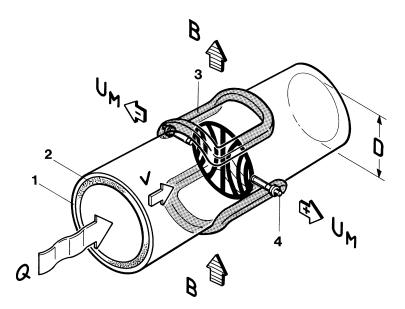
Through a meter tube provided with an insulating lining a liquid flows at velocity v and a flow rate Q, producing a measuring-circuit voltage Um at the two electrodes at right angles to the direction of flow. The size of this measuring-circuit voltage is proportional to the mean flow velocity and the volume flow rate.
