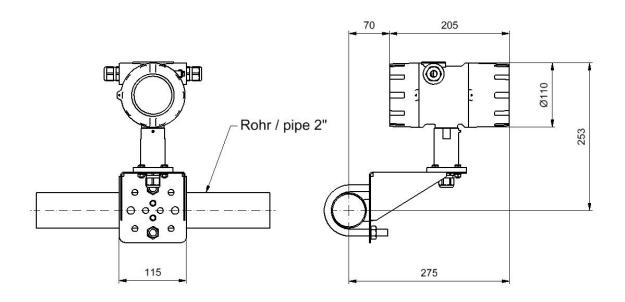
SG2 transmitter housing vertical pipe mounting
