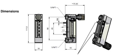
The threaded pins M4 are only mounted if the option "Wall Mounting" has been selected.
