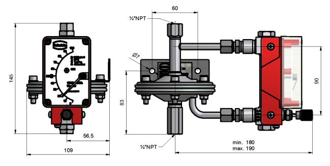
KDS-R...-N with 1/4" NPT (F) connection as outlet pressure controller version
