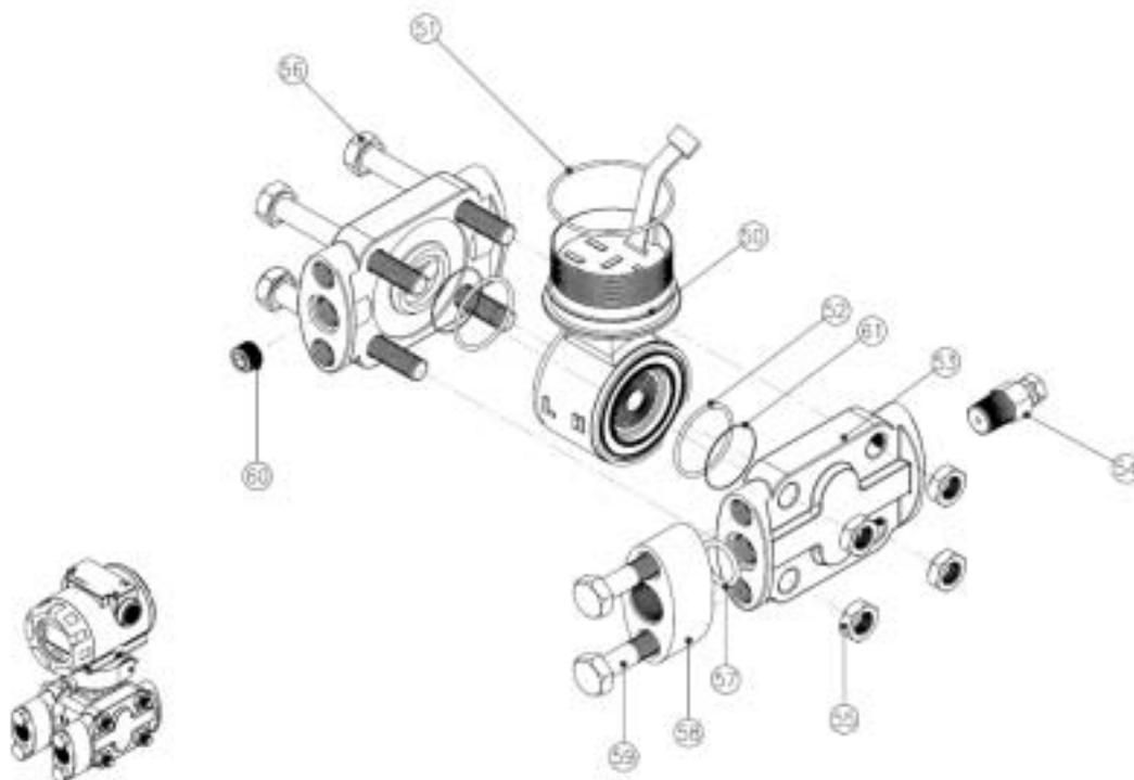
Figure 2-5. Model PAD Exploded View (Sensor Module-H)
