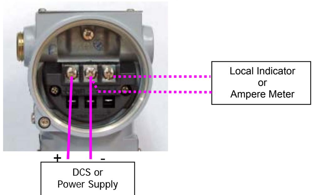
Figure 5-3 Picture of Terminal Board of Transmitter
