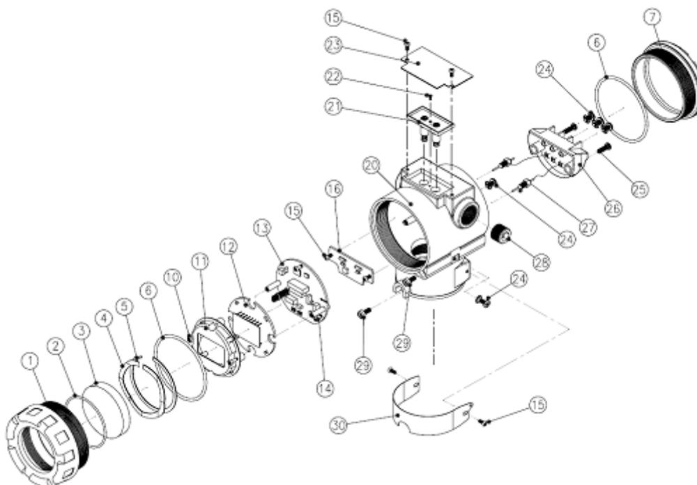
Figure 2-1. Model PAD Transmitter Exposed View (Housing)
