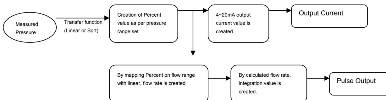
**Note:** PAD-F measures the flow rate by using differential pressure. It cannot compensate the changes in operating temperature and static pressure.
