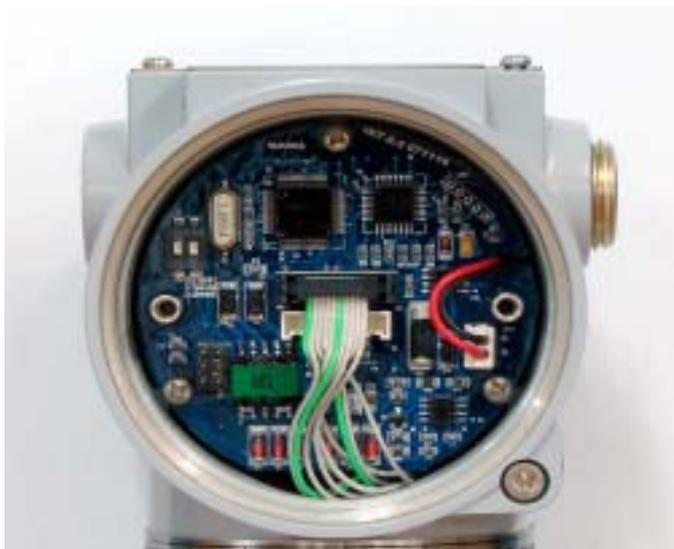
Figure 7.3 Structure of Electronics Module inner Transmitter
