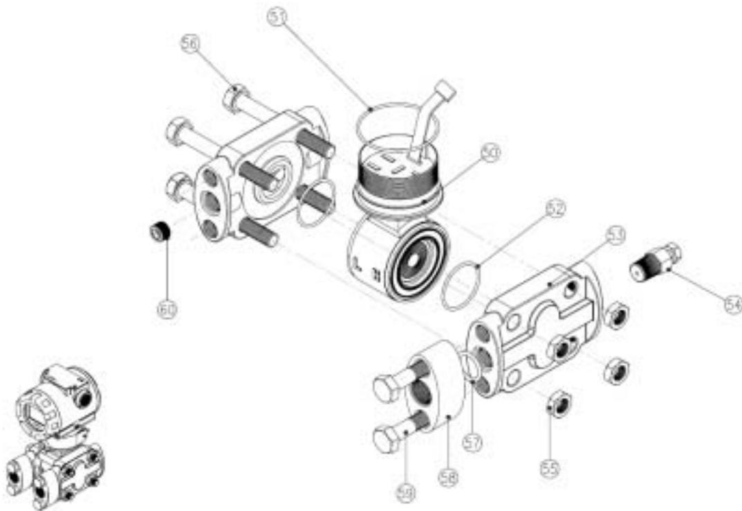
Figure 2-3. Model PAD Exploded View (Sensor Module-D,G)
