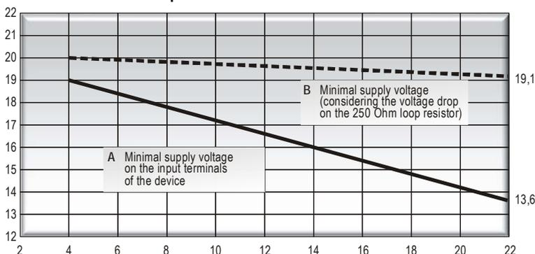
**A:** minimal supply voltage on the input terminals of the device
