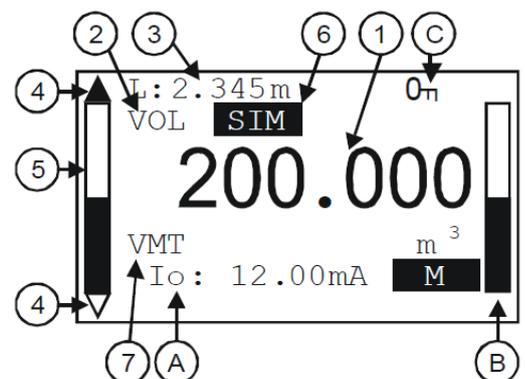
6. Indication of Primary Value simulation. In this case the display and output show the values of the simulation and not the measured values.
