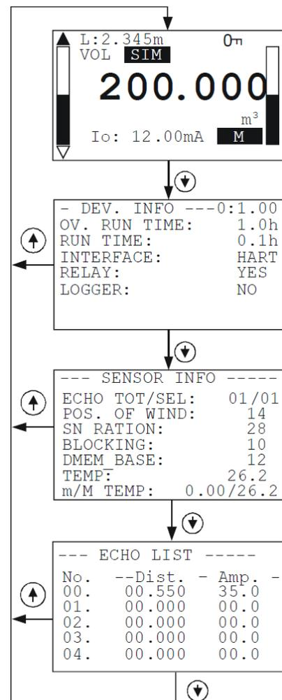
The informative screen returns back to main screen after 30 seconds. By pressing the  $\uparrow$  button the user can return to the main screen any time. Pressing the  $\text{\textcircled{E}}$  button in any of the screens the user can enter the main menu. After exiting the menu always the main screen will be shown.
