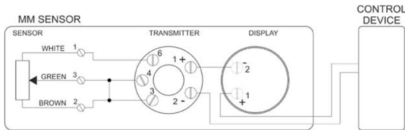
**13.5 Wiring diagram with touch screen LCD display type R**
