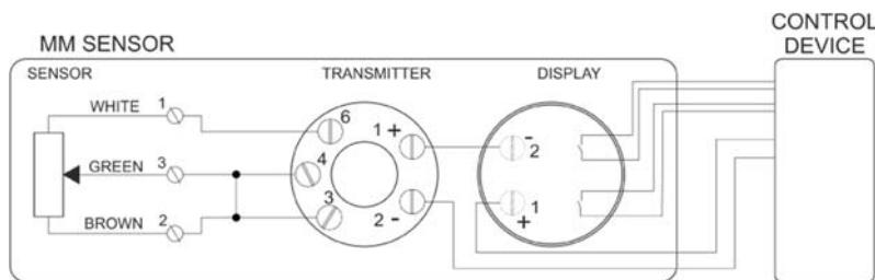
**13.6 Wiring diagram with LED display type E**
