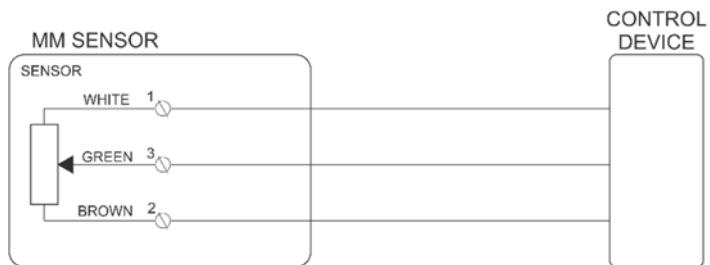
**13.3 Wiring diagram with transmitter**
