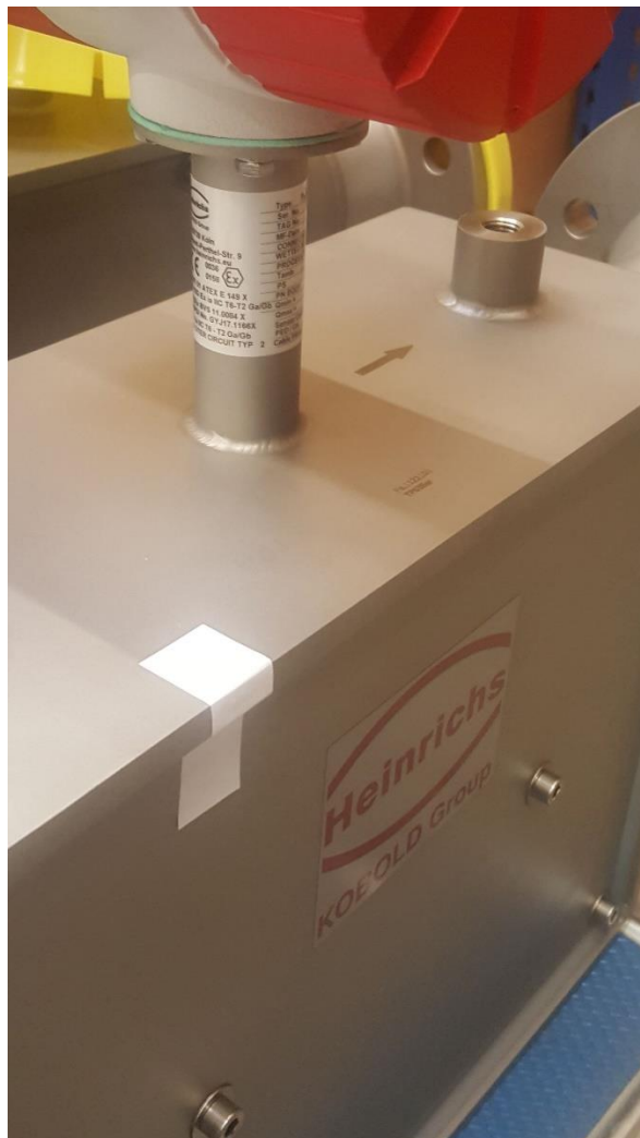
Image 3 and 4: Seal securing the sensors removable lid
