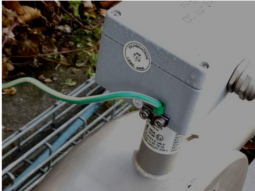
Image 2: Seal securing the sensors terminal box lid
